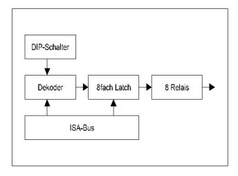
The block diagram of the board IO 1335 is shown in figure 1.
